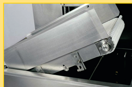
RET-A-4 / RET-A-4-11. Raising of the conveyor belt to facilitate cleaning of interior of tank.
