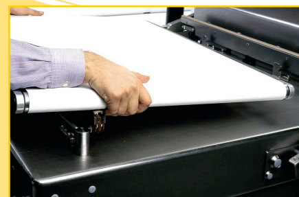
EVD-A-20. Easy removal of the conveyor belt for cleaning.
