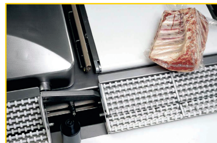
EVD-A-20. Automatic expelling of product at the end of the vacuum packing cycle.
