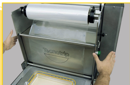
Two button activation for automated entry in the drawer. The exit is done automatically when the cycle is finished (convenient for cold product packaging).
