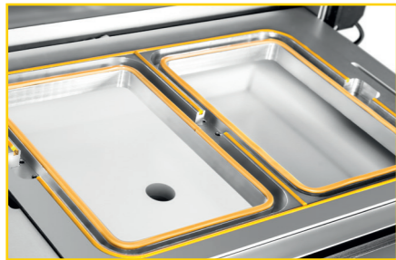
Perimeter cut and seal. Entry and exit using the automated drawer in the TSB-A-100 or done manually in the TSB-100.
