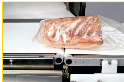
PA-9-11. The automatic leveling of the two belts facilitates the movement of the product, ensuring a perfect placement.
