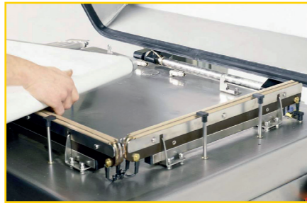
EVA-9-11. Easy removal of the conveyor belt for cleaning.
