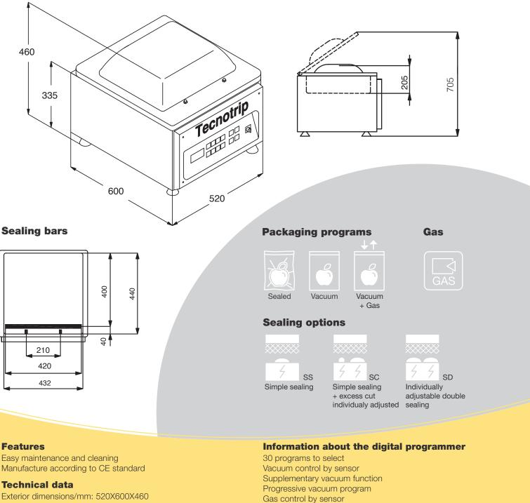
Chamber dimensions/mm: 430X440X205 Cycles/min: 2/3 Power/Kw: 0,75 Electrical connection: 220V 50H/60Hz 1ph Weight/kg: 60
